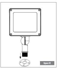
AFTER INSTALLATION. PLEASE: • CHECK IF THE LIGHTING FIXTURE IS MOUNTED FIRMLY. • CHECK IF THE WIRES ARE CONNECTED PROPERLY. • TURN ON THE POWER.
